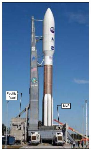
Figure 13. Atlas V, MLP and Facility Vault
